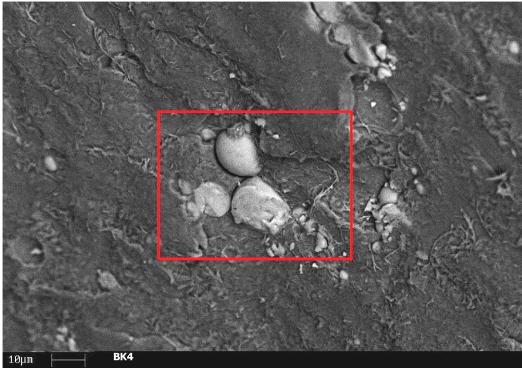
Fig. 2. Particles of octaphenyl-POSS in PA6 matrix after the in situ hydrolytic polymerization of CL (back scattering image).
